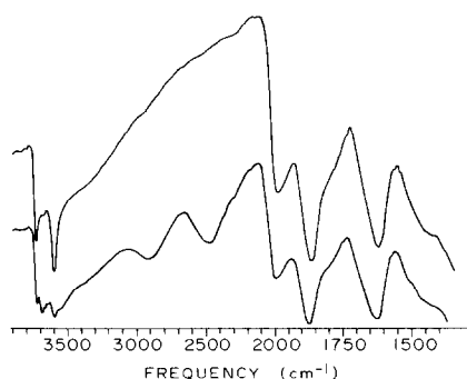
FIG. 3. Transmission infrared spectra for \text{H-ZSM-5} with and without adsorbed water at 300\text{ K} . The 3605\text{-cm}^{-1} peak is severely attenuated, even though the water coverage is \sim 0.7 molecules/cation.
